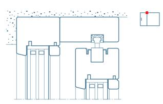
Wood and image only: the hardware disappears on the frame The sliding top guide has been inserted into the frame to hide very functional element.
