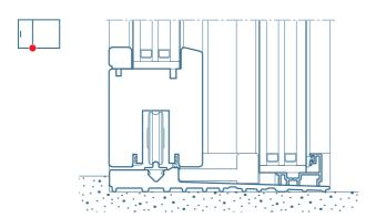
Leaving space to the glass: a room without bounds The lower transom of the fixed sash has been eliminated. The glass and the external environment become the center of the room.
